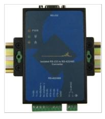
With the RS-232/RS-422 converter it is possible to control the sensors through an industrial interface. Consequently, it is possible to control D-Series devices which are placed remotely (up to 1200 m).
